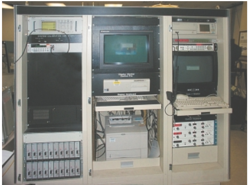
Figure 1. The Pratt & Whitney Rotating Machinery Analysis System. The VME cage is accessible from the rear of the rack. (Courtesy of Pratt & Whitney)
