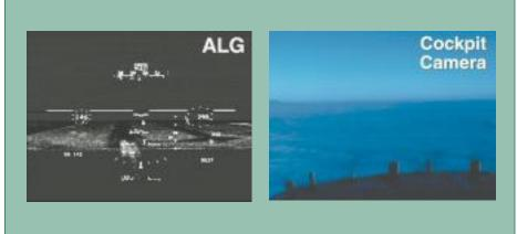
Figure 1. View from the cockpit with and without ALG (Courtesy of BAE Systems)
