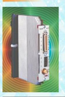
Intended for Pentek's VIM-compatible processor boards, Model 6215 is a VIM-2 module that includes eight 16-bit sigma-delta A/D converters, with 4.7 kHz to 234 kHz sample rate. Two of these modules can fit on a processor board to provide 16 A/D channels which utilize all four processors while occupying just one VMEbus slot.
