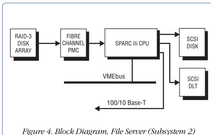
Figure 4. Block Diagram, File Server (Subsystem 2)
