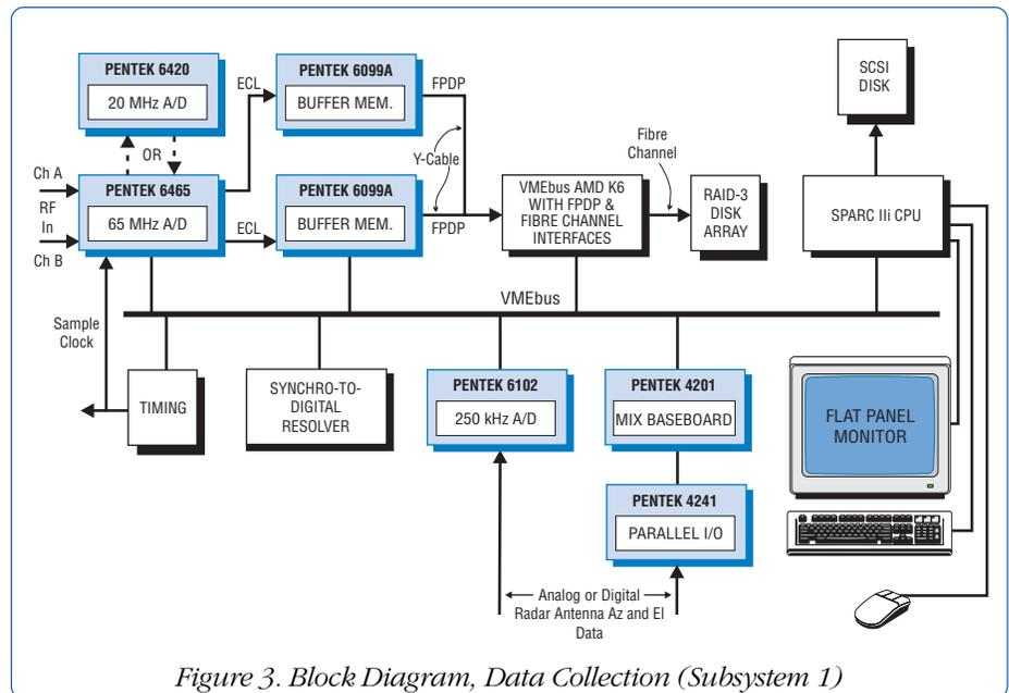
Figure 3. Block Diagram, Data Collection (Subsystem 1)
