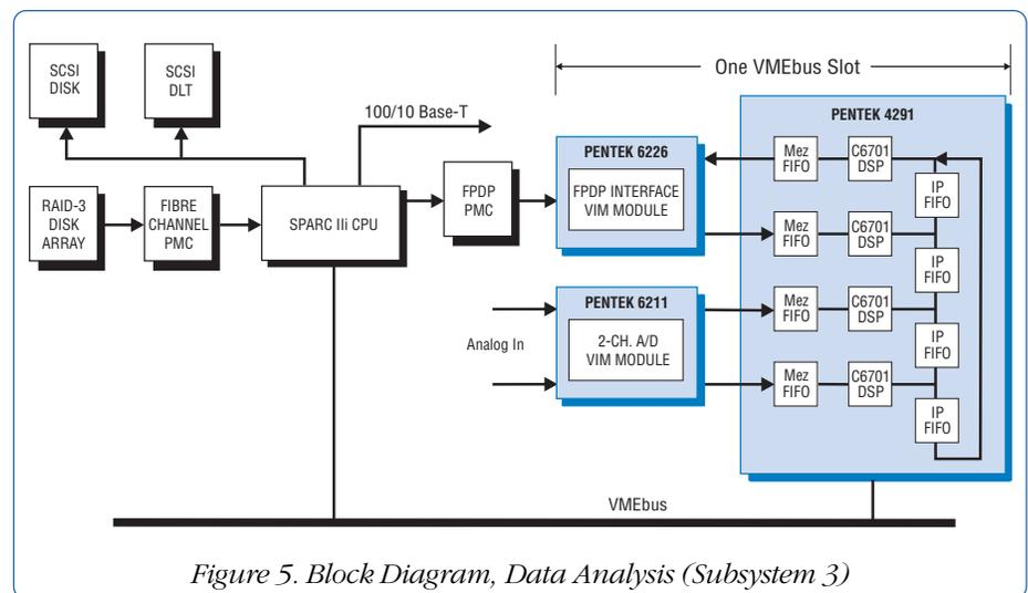
Figure 5. Block Diagram, Data Analysis (Subsystem 3)
