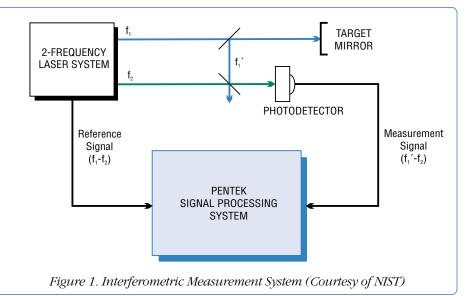
The Atomic Displacement Metrology Project (ADM) at NIST is an effort to extend the technology of laser-based distance measuring interferometers into the picometer domain. Just so we can keep our units in the proper perspective,
