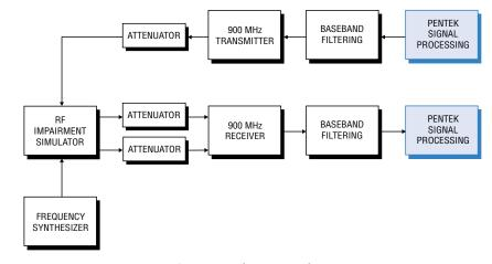
Figure 4. Hardware Configuration for Measurements
