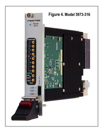
technology and features four 200 MHz 16-bit A/Ds and four multiband digital downconverters. It is equipped with dual XMC connectors, each capable of supporting 8 lanes of gigabit serial links. The standard product uses one of these connectors for a PCIe Gen 3.0 x8 interface, delivering a peak data transfer rate of 8 GB/sec through the 3U VPX carrier to the VPX backplane.
