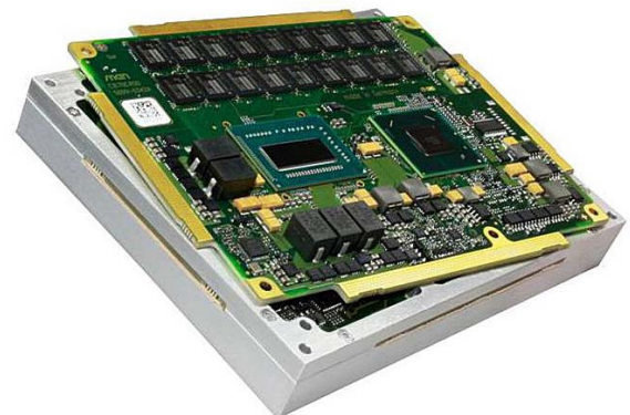
Figure 1. VITA 59 Rugged Com Express module adds thermal tabs to the sides of COM Express boards to pull heat out to a rugged aluminum frame (Courtesy of Men Micro)
