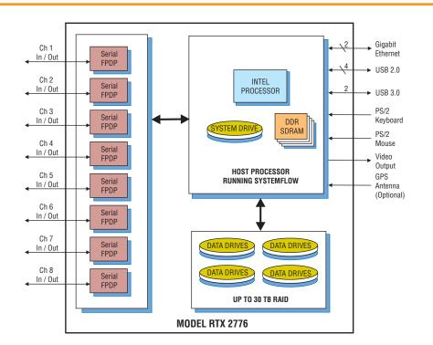
Built on a server-class Windows 7 Professional workstation, the RTX 2776 allows the user to install post-processing and analysis tools to operate on the recorded data.
