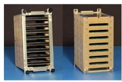
Figure 5. Front and rear view of the QuickPac canister showing the eight SSDs inside.
