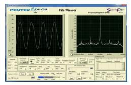
Pentek's <u>SystemFlow Simulator</u> for Talon analog and digital recording systems includes a virtual recorder server application that simulates disk and I/O transactions for a complete and realistic recording environment.
