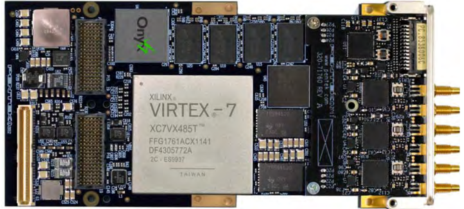
Figure 6. Pentek Onyx Model 71760 Four-Channel A/D XMC Module
