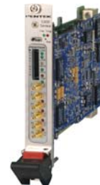
Model 53630: 1 GHz A/D and D/A - 3U VPX
