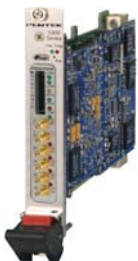
Model 53621: Model 71620 with Wideband DDCs and Interpolation Filter - 3U VPX
