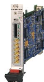
Model 53630: 1 GHz A/D and D/A - 3U VPX
