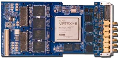
Model 71620: Transceiver, three 200 MHz A/Ds, DUC and two 800 MHz D/As - XMC
