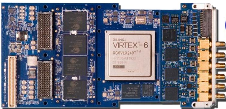
*Pentek XMC Software Radio Board with Virtex-6 FPGA*
