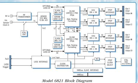
320 MB/sec. One port per FPGA is attached to the 6821 front panel, while the second is available on an optional second-slot panel. A data demultiplexing mode splits the data stream between each pair of FPDP ports reducing data rates by a factor of up to eight to support slower FPDP devices. Additional LVDS data I/O is available through either the VMEbus P2 connector or the optional second-slot front panel.
