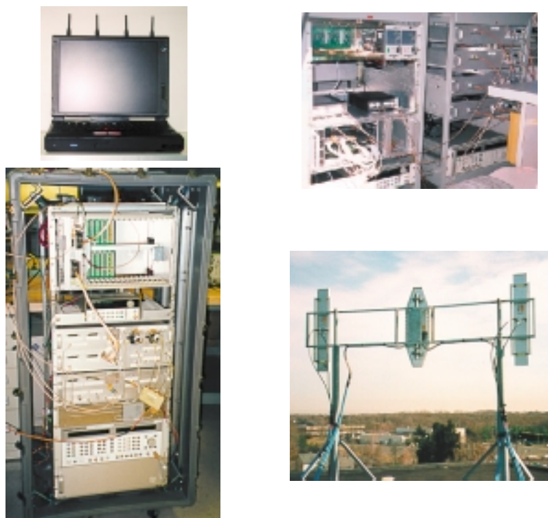
Figure 2. Upper : Transmitter with four antennas on a laptop and the 1900 MHz coherent transmitters. Lower : The four receivers with real-time baseband processing and the rooftop antennas (Courtesy of AT&T Labs-Research).
