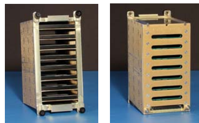
Figure 5. Front and rear view of the QuickPac canister showing the eight SSDs inside.
