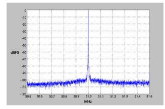
${\rm f_{in}} = 69~{\rm MHz}, \ {\rm f_s} = 100~{\rm MHz}$  Phase Noise @ 100 kHz = -102 - 10\*log(610) = -129.8 dB/Hz
