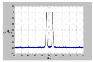
$f_1 = 69.5 \text{ MHz}, f_2 = 70.5 \text{ MHz}, f_s = 100 \text{ MHz}$
