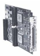
One VIM-2R plus one VIM-2 module may be attached to a 4290 or 4291 processor boards.
