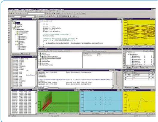
menu-driven graphical interface for the debugging and networking capabilities of SwiftNet. It integrates system debuggers, signal probes, and other tools into one Windows environment that supports TI's C6000 DSP processor family.
