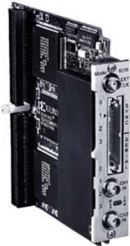
Two VIM-2 modules may be attached to VIM-compatible processor boards.
