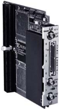
Two VIM-2 modules may be attached to VIM-compatible processor boards.
