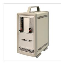
The 8257 is a low-cost 3U VPX chassis ideal for developing applications on Mercury's 5550 or 5553 Quartz® RFSoC boards. Providing power and cooling to match the 5950 and 5953 in a small desktop footprint, the chassis allows access to all required interfaces on the 5950 and 5953 front panel and the 5901 rear transition module. The 8257 can be configured with optional rear-panel dual MPO optical connectors to support the dual 100 GigE interfaces on the 5950 and 5953.
