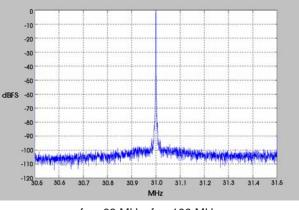
$f_{in} = 69 \text{ MHz}, f_s = 100 \text{ MHz}$ Phase Noise @ 100 kHz = -102 - 10\*log(610) = -129.8 dB/Hz
