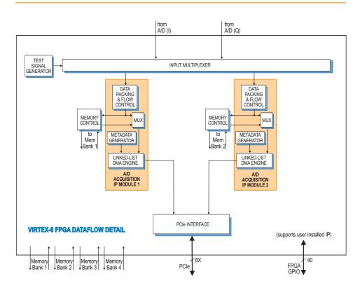
➤ Each QDRII+ SRAM bank can be up to 8 MB deep and is an integral part of the module's DMA capabilities, providing FIFO memory space for creating DMA packets. For applications requiring deeper memory resources, DDR3 SDRAM banks can each be up to 512 MB deep. Built-in memory functions include multichannel A/D data capture, tagging and streaming.
