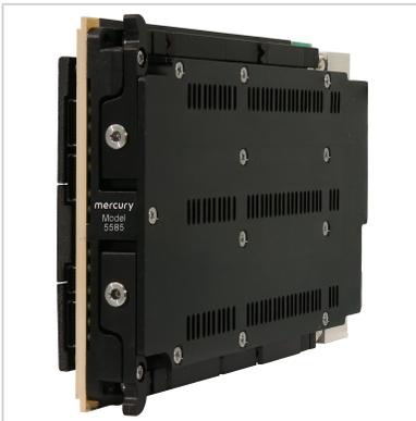
**The 5585 SOSA aligned 3U OpenVPX board is an 8-channel, high-speed data converter with programmable DDCs (digital down-converters). It is suitable for connection to HF or IF ports of a communications or radar system.** Its built-in data capture feature offers an ideal turnkey solution as well as a platform for developing and deploying custom FPGA-processing IP.
