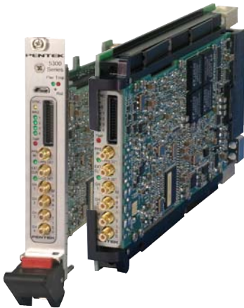
Model 5350 commercial (left) and conduction-cooled version
