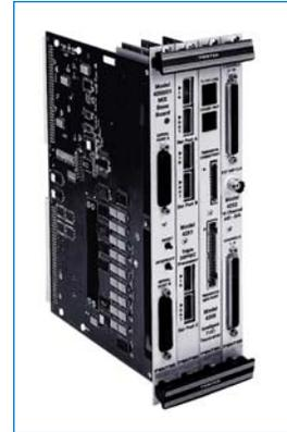
*16-channel data acquisition and signal analysis system with T1/E1 interface fits in just four VMEbus slots. System consists of a 4200A MIX Baseboard, a 4257 Dual C40 Coprocessor, a 4259 T1/E1 Transceiver and a Model 4252 16-channel A/D and D/A Converter.*
