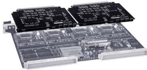
Pentek VIM modules attach directly to the processor board through the I/O connectors. Shown here are two Model 6223 Comm Port Adapter VIM-2 modules in the process of being plugged into a Model 4291 Quad C6701 Processor board as viewed from the rear of the board. Two different modules may be used to provide more I/O functions.
