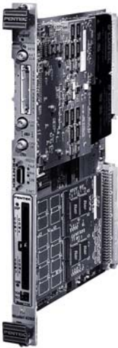
The Model 4292 Quad C6203 Processor board. A Model 6210 VIM module is attached to the upper part of the board and a Model 7110 PMC module to the lower part of the board.
