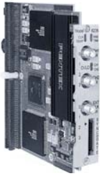
Model 6235 is a dual wideband digital receiver VIM-2 module; it includes two A/Ds and one FPGA for custom signal processing.
