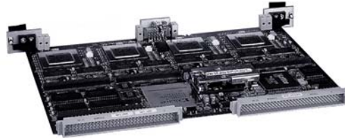
The Pentek Model 4291 Quad C6701 Processor board, as viewed from the rear of the board, without any VIM modules attached.
