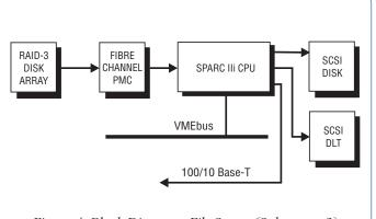
Figure 4. Block Diagram, File Server (Subsystem 2)
