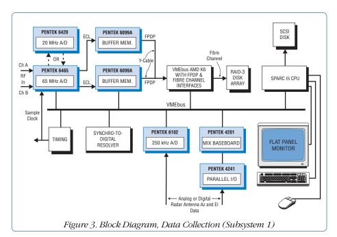
stores the data to the RAID-3 disk array which has 72 GB storage capability. The File System has the ability to access disks at 50 MB/sec.
