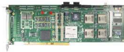
The T2-PCI board from Bittware, in Concord, N.H., uses a Xilinx Virtex-II Pro FPGA for I/O and routing but uses four TigerSHARC 201 DSPs from Analog Devices for most of the computing.
