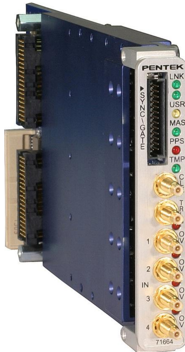
Figure 6: Model 71664 Quad 200 MHz ADC and multi-band DDC XMC module delivers VITA 49.0 packet streams across
