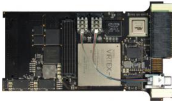
Figure 3. Pentek Model 5973 3U VPX Virtex-7 FMC carrier uses Samtec FireFly™ Micro Flyover delivering 12 optical fiber pairs to the proposed VITA 66.4 backplane I/O. (Image courtesy Pentek)
