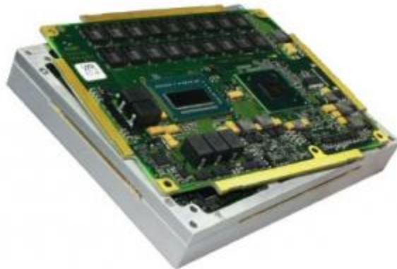
Figure 1. VITA 59 Rugged COM Express module adds thermal tabs to the sides of COM Express boards to pull heat out to a rugged aluminum frame. (Image courtesy MEN Micro)
