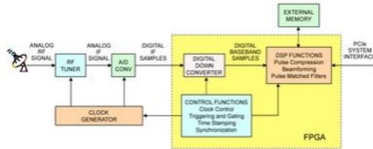
**Figure 2:** Functional blocks of a typical FPGA-based radar receiver
