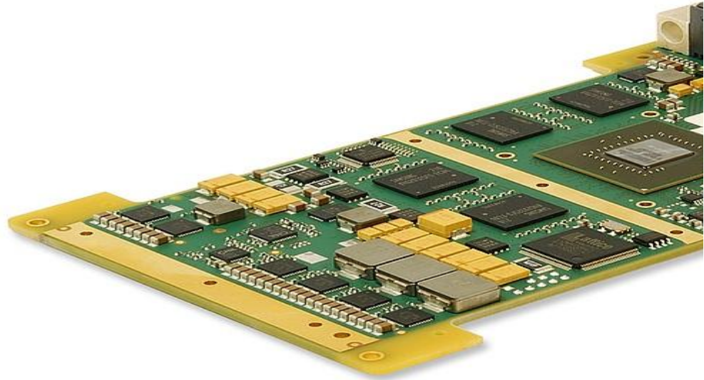
Figure 1: The GRA113 leverages commercial NVIDIA technology on a form factor aimed at use in rugged radar and electronic warfare applications. Photo courtesy of Abaco Systems.
