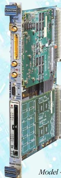
*Model 4292 shown with Model 6210 VIM module and Model 7110 PMC Module*
