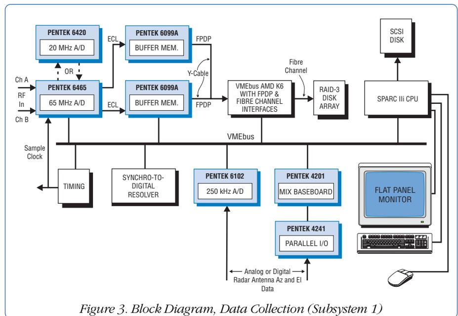
Figure 3. Block Diagram, Data Collection (Subsystem 1)
