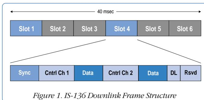
Figure 1. IS-136 Downlink Frame Structure
