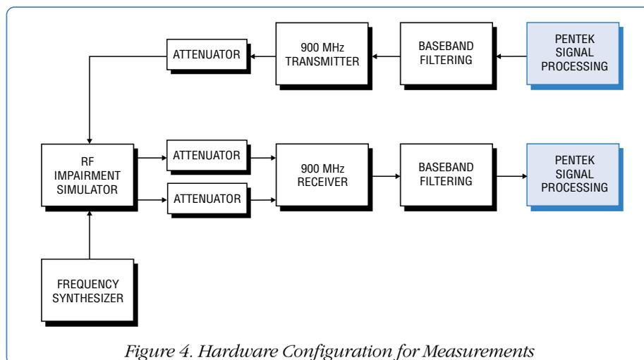
Figure 4. Hardware Configuration for Measurements
