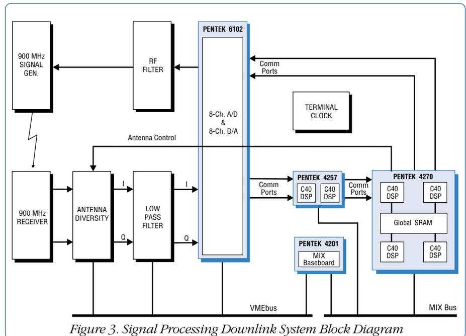
Figure 3. Signal Processing Downlink System Block Diagram
