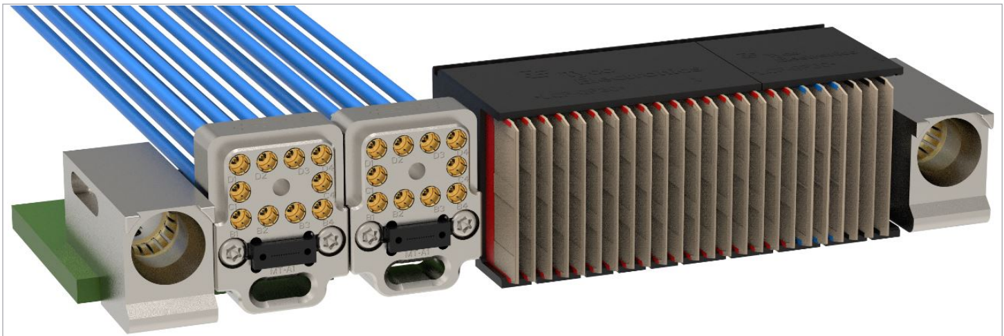
Figure 2. Rear view of 3U OpenVPX Module with two VITA 67.3D backplane connectors, each with 10 coaxial RF signals and 24 optical lanes. Courtesy TE Connectivity
