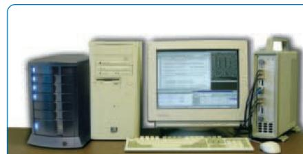
*Commercial off-the-shelf (COTS) System RTS 2501 Scalable Modular Data Acquisition and Processing System*
