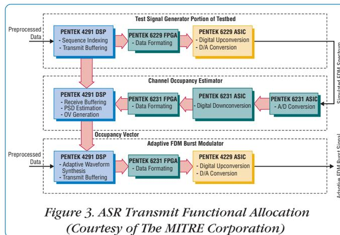
Figure 3. ASR Transmit Functional Allocation (Courtesy of The MITRE Corporation)
