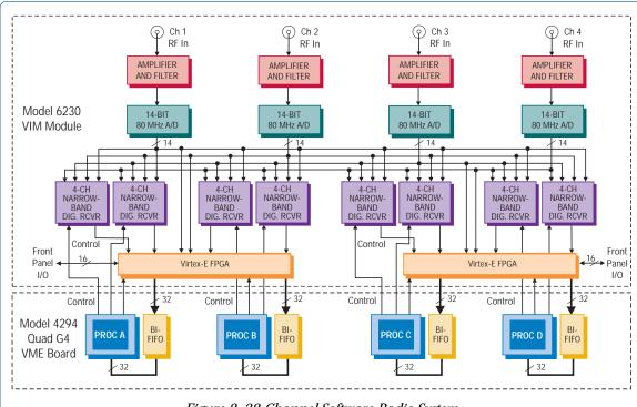
Figure 2. 32-Channel Software Radio System
