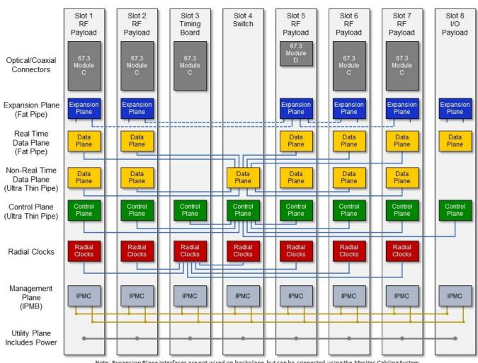
\_\_\_\_ Note: Expansion Plane interfaces are not wired on backplane, but can be connected using the Meritec Cabling System
