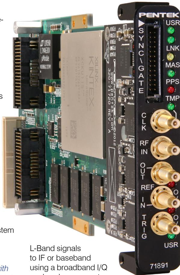
L-Band signals to IF or baseband using a broadband I/Q analog downconverter followed by 123 MHz low pass anti-aliasing filters. The two analog tuner outputs are digitized by two Texas Instruments ADS5474 400 MHz 14-bit A/D converters to capture the full 123 MHz bandwidth.
