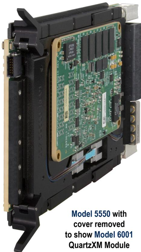
**Model 5550 with cover removed to show Model 6001 QuartzXM Module**
