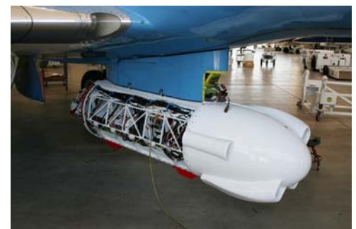
Another close-up photograph of the UAVSAR Pod with the electronics cover removed. (Photo courtesy of DFRC)
