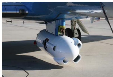
Close-up photograph of the UAVSAR Pod attached to the underside of the aircraft. (Photo courtesy of DFRC)
