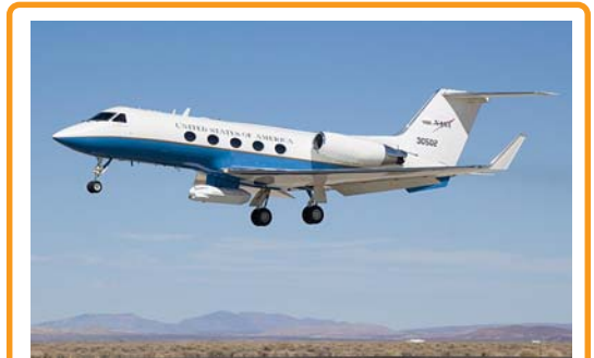
Figure 1. The UAVSAR pod is attached to the underside of the aircraft. (Photo courtesy of DFRC)
