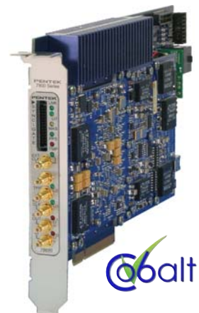
Figure 2. The Pentek Cobalt 78690 PCI Express board uses an LNA to boost L-Band signals between 925 and 2175 MHz, as well as a programmable-gain RF amplifier for 60 dB of overall gain control
