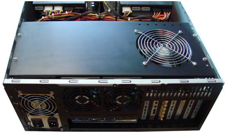
Figure 4. A top-mounted 120 mm fan blows air down onto expansion cards
