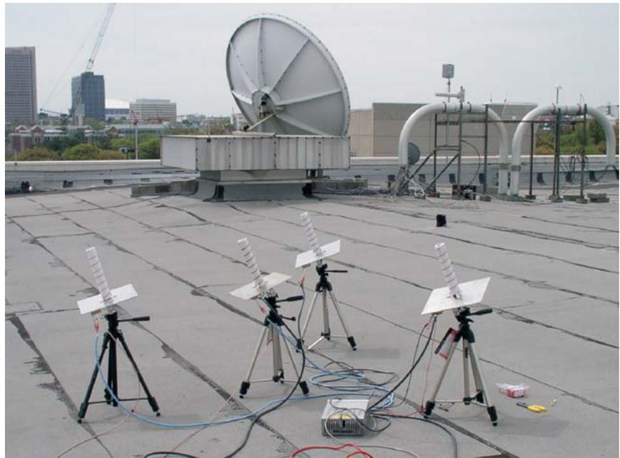
Figure 1. Four Helical Antennas Receiving the Signal from EO-1
