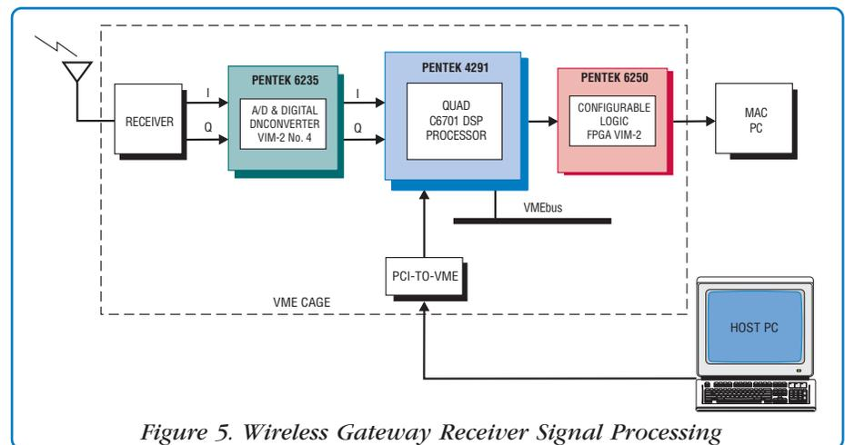
Figure 5. Wireless Gateway Receiver Signal Processing
