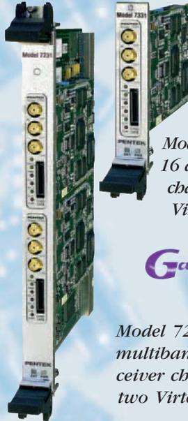
*Model 7331 offers 16 digital receiver channels with a Virtex-II FPGA.*
