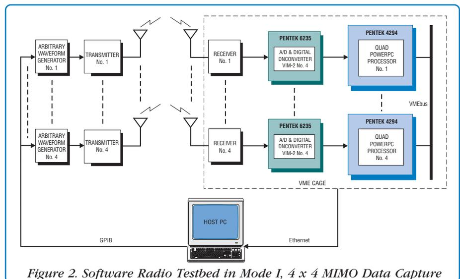
Figure 2. Software Radio Testbed in Mode I, 4 x 4 MIMO Data Capture
