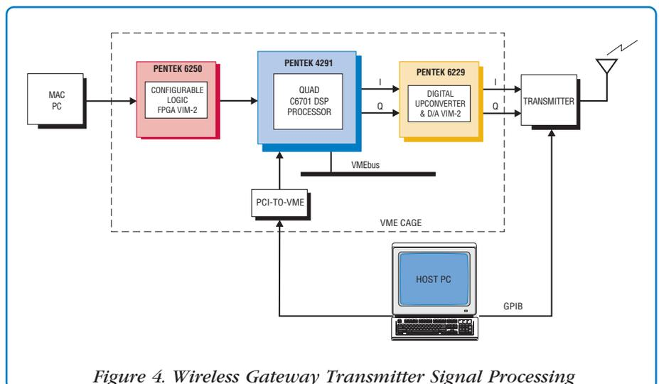
Figure 4. Wireless Gateway Transmitter Signal Processing
