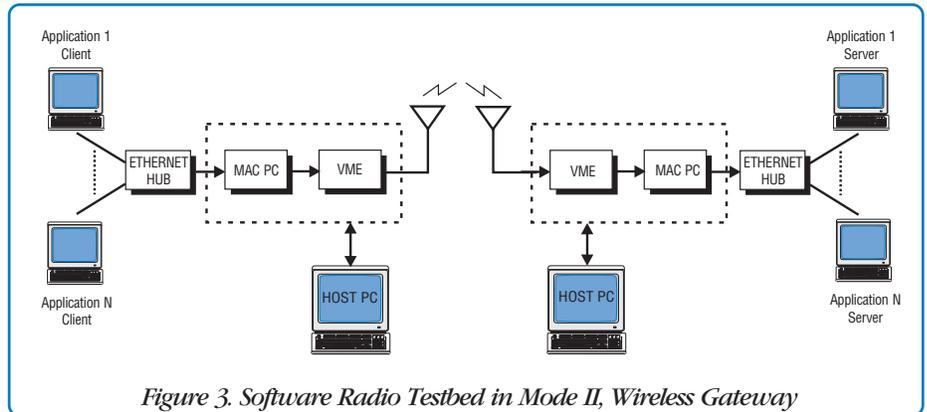
Figure 3. Software Radio Testbed in Mode II, Wireless Gateway
